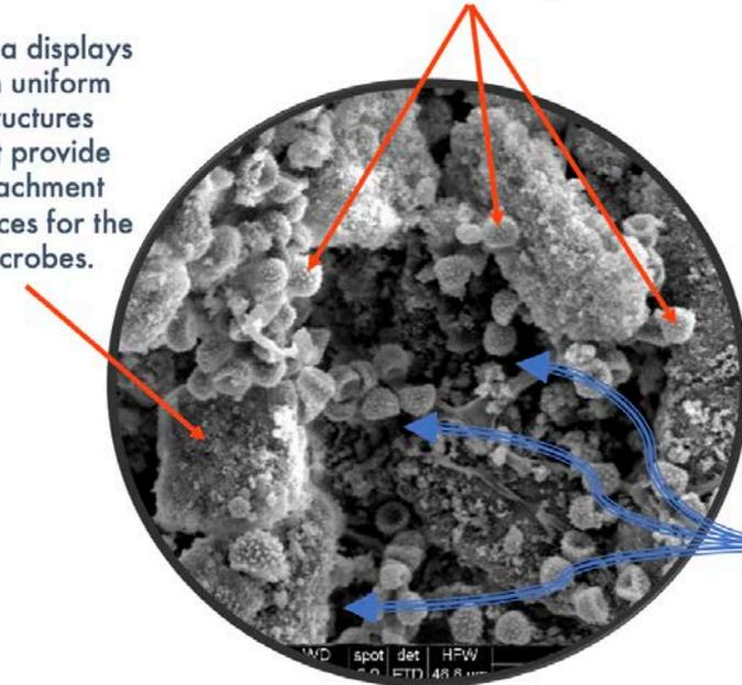
Soluble materials are adsorbed and diffused into the particle, feeding the microbes.
